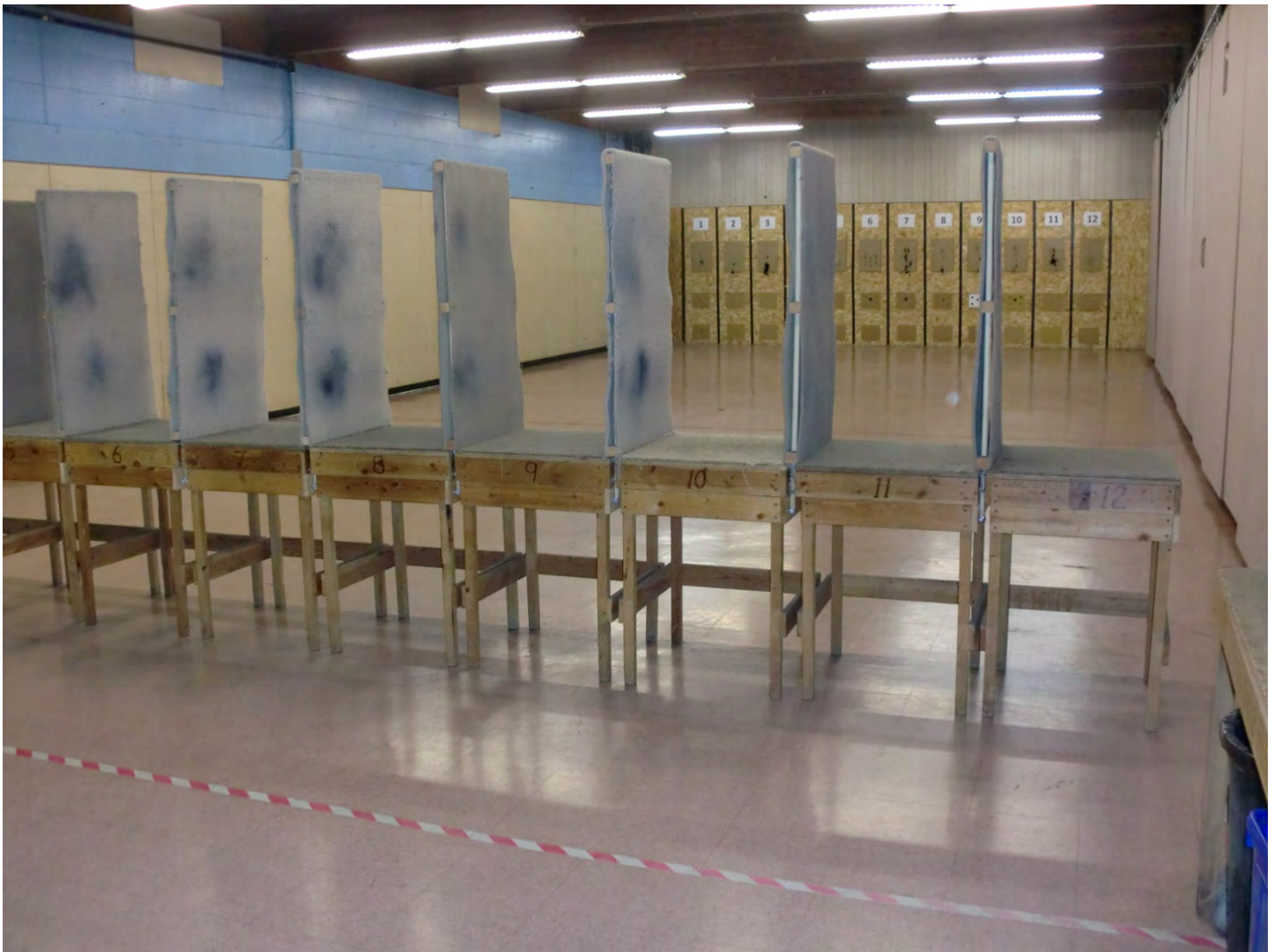
Figure 1 - The indoor range - 12 shooting positions with carpeted benches and vertical shields to protect adjacent shooters from fired and ejected cases. Note that shooting positions #1 and #12 are marked for ROs and designated experienced shooters only as they are adjacent to the wall. The new acoustic sound panels are visible on the right side wall.
